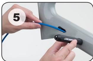
**EN** Use the main magnet (A) to guide the hydraulic hose along the frame tube.
