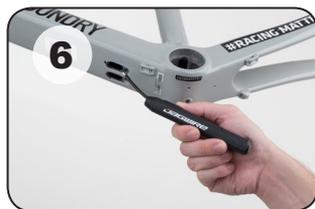
**EN** Extend the flexible magnet (B) using the slider, and insert into the exit port on the frame.
