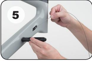
**EN** Use the main magnet (A) to guide the inner cable along the frame tube.
