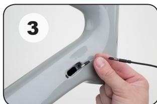
**EN** Insert the E-Tube wire into the frame, leading with the magnetic end of the flexible wire (F).
