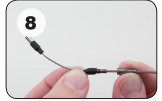
**EN** Unthread the E-Tube fitting (H) from the flexible wire (F), and remove from the inner cable.
