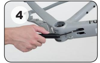
**EN** Use the flexible magnet (B) to draw the housing out of the frame.
