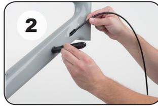
**EN** Use the main magnet (A) to guide housing along the frame tube.
