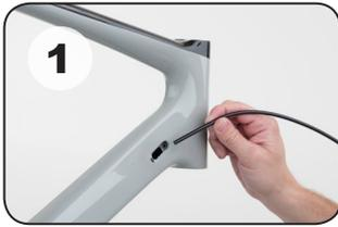
**EN** Insert the cable housing into the frame.
