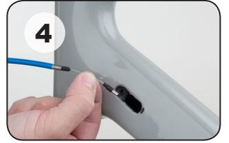
**EN** Insert the hydraulic hose into the frame, leading with the magnetic end of the flexible wire (F).
