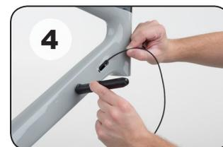
**EN** Use the main magnet (A) to guide the wire along the frame tube.
