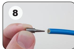
**EN** Unthread the flexible wire (F) from the hydraulic hose fitting (G), and unthread the fitting (G) from the end of the hose. Use a hydraulic hose cutter to remove 10mm of hose before inserting a needle.
