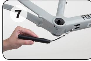
**EN** Use the flexible magnet (B) to attach to the magnetic end of the flexible wire (F), and remove from the frame.
