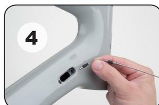
**EN** Insert the inner cable into the frame, leading with the magnetic end of the flexible wire (F).
